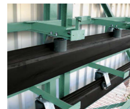
High-care transport thanks to enclosed belt design
